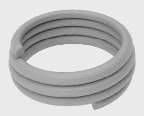
Ferrocell 316 is a closed cell polyethylene in round strip shape suitable for using as a sub joint (Backing rod) to polyurethane, silicone or acrylic joint sealant application. Ferrocell 316 has a high recovery property, medium density, light weight, good flexibility that can resistant to a general movement of precast concrete wall joint.
