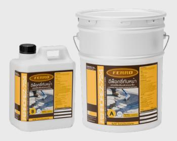
Ferrorez 724 is a 2 component polyamide epoxy resin (solvent base). Use for coating upcon smooth concrete surface a high gloss, waterproof, oil, chemicals and acid resistant properties. Ferrorez 724 has a high viscosity that can penetrate into smooth concrete surface such as dry shake floorhardener floor surface. Ferrorez 724 is suitable for interior use in area of carpark, light industrial floor.
