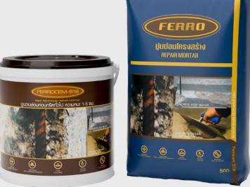
Ferrocem 518 is a repair mortar with microfiber suitable for repairing an imperfect concrete surface or honeycombs. Ferrocem 518 has a high adhesion, compressive strength and also easy for patching with thixotropic property. Ferrocem 518 can be used in patching both in vertical and horizontal works such as concrete beam and column repairs.
