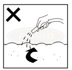
CASE 2 Old or existing concrete surface are coated with transparent film such as curing compound or oil contaminants.
